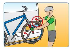
When your bike is loaded, lift the tire hook over the front tire to secure it in place.
